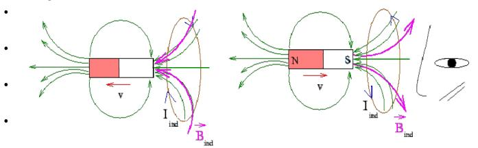
In the figures the loops are perpendicular to the plane of the page. The direction of induced current is as seen towards the loop from the right. Note that the magnetic field set up by the induced current tends to increase the flux in the case where the magnet is moving away from the loop and tends to decrease it in the case where it is moving towards the loop,
