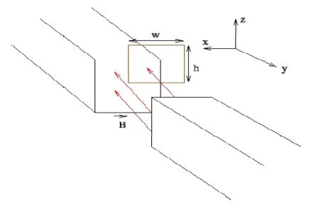
(a) Find the current in the loop when the speed of the loop is  $\mathcal{V}$  and (i) it is partly inside and partly outside the field region (ii) it is wholely inside the filed.
