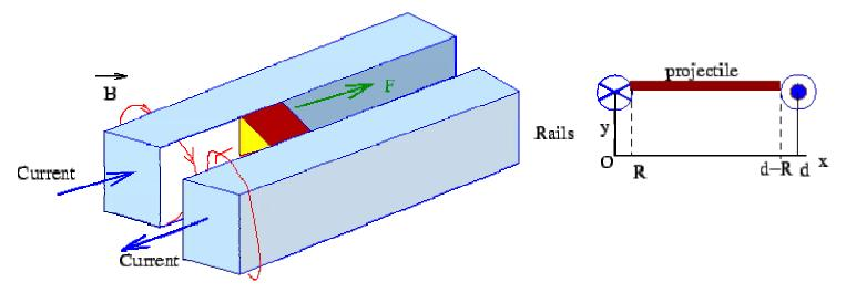
In the figure shown, the radii of cross section of the rails are R each and the separation between them is d. The fields due to both the wires are in the -y direction, so that the force  $I \vec{dl} \times \vec{B}$  acts along the direction, parallel
