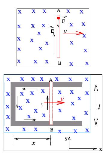
The fixed positive ions in the conductor are immobile. However, the negatively charged electrons experience a Lorentz force  $- | \varepsilon | \vec{v} \times \vec{B} = - | \varepsilon | vB\hat{j}$ , i.e. a force along the -y direction. This pushes the electrons from the end A to the end B, making the former positive with respect to the latter. Thus an induced electric field is established in the
