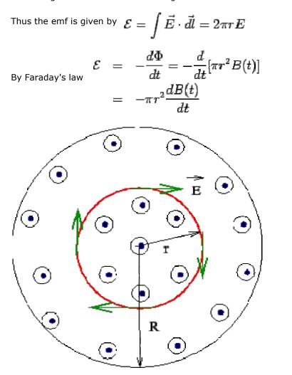
Equating these, we get for  $r \leq R$   $E = -\frac{r}{2}\frac{dB}{dt} = -\frac{B_0\omega}{2}r\cos\omega t$ For r > R, the flux is  $\Phi = \pi R^2 B(t)$ , so that  $\mathcal{E} = -\frac{d\Phi}{dt} = -\pi R^2 \frac{dB}{dt}$ and the electric field foir r > R is  $E = -\frac{R^2}{2r}\frac{dB}{dt} = -\frac{B\omega R^2}{2r}\cos\omega t$
