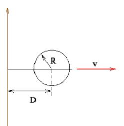
(Hint : Consider the field at an element of area  $r dr d\theta$ . The distance of the element from the wire is  $D + r \cos \theta$ . Calculate the flux by integrating from r = 0 to R and from  $\theta = 0$  to  $2\pi$ . Use :  $\int_{0}^{2\pi} \frac{d\theta}{D + r \cos \theta} = \frac{2\pi}{\sqrt{D^2 - r^2}}$ (Answer  $\mu_0 I v (D/\sqrt{D^2 - R^2} - 1)$ )
