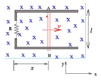
The force acting on the sliding conductor is  $F=Iec{L} imesec{B}=-rac{B^2l^2v}{R}\hat{\imath}$
